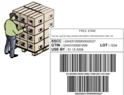
→ **GS1-128** is a linear bar code symbology. **Data Matrix** is a 2D symbology. They are both able to carry information using GS1 Application Identifiers, which are defined by GS1 and enable the bar coding of information such as product identification (GTIN), expiry date, shipping information, etc. The bar code used is according to data required for the business application, as well as the size of the packaging.
