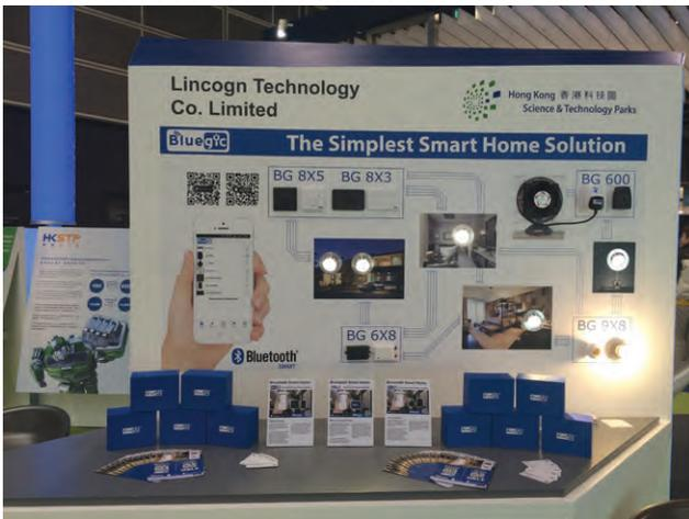
Lincogn Technology, which specializes in Bluetooth R & D and manufacturing of various related electrical accessories, has developed Bluetooth Smart Home to tap potential demand in the smart home market. Its products are designed to replace the existing wall switches in ordinary homes, with no configuration required, because these Bluetooth-enabled items can be controlled by a proprietary app available for downloading on smartphones.
