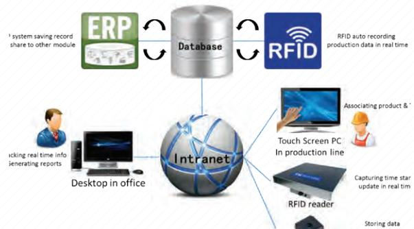
This system is integrated with the factory's Enterprise Resource Planning (ERP) system to automatically generate records of defective or partially finished products, analyze the collected data and produce precise production records. These reports provide the traceability and visibility that management needs, in order to take immediate action in contingency situations such as urgent order placements or unforeseen machinery downtime.
