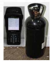
storing a range of data (including cylinder ID, SAP batch number, article number and inspection date) are used.
