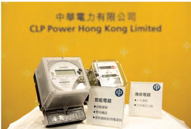
Leveraging on IoT technology, a mEnergy programme has been developed by CLP to provide residential and corporate customers with regular energy consumption information. In fact, the entire Advanced Metering Infrastructure of the electricity provider has been reconfigured to realize the IoT Concept. Devices, such as smart meters and routers, are integrated with billing and other systems, which can be connected to the customers' smartphones via the Internet.
