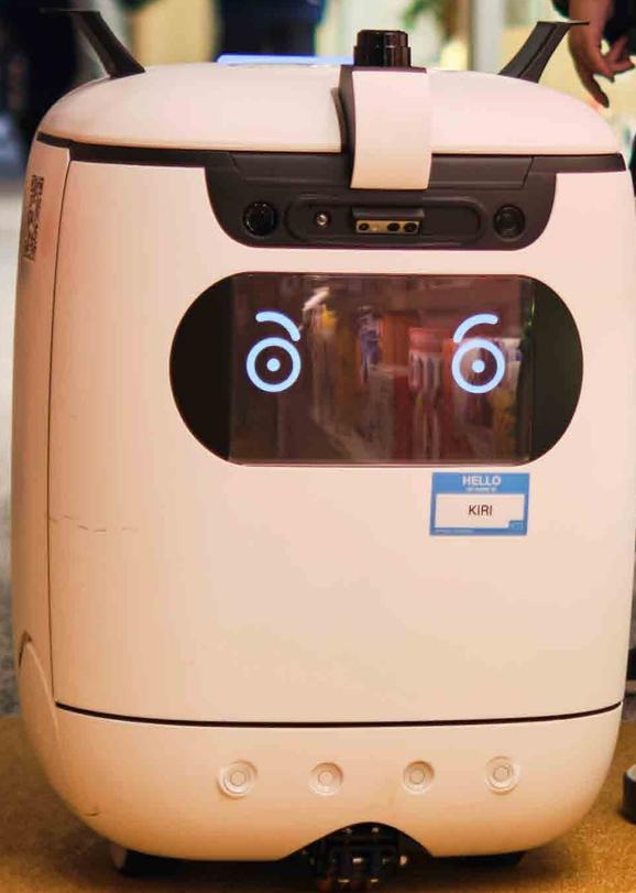
Safeguarding the health and safety of customers has been a key priority for retailers during the COVID-19 pandemic. Hong Kong-based start-up Rice Robotics has introduced disinfection robots, delivery robots and security robots at several of the city's major shopping centres. The robots can operate elevators, charge themselves and navigate through indoor spaces without help. The Jasmine disinfection robot (pictured here at the K11 Musea mall) disinfects 12 hours per day from 10 am to 10pm.
